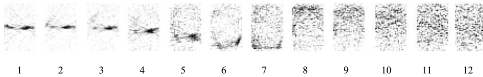
FIG. 10. PET images showing the spread of a pulse initially positioned in the middle of the fluidized bed. The time in seconds is given below the images. Details of the experimental and analysis method are given in Ref. [8].
